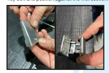
STEP 4: Insert acrylic screen and tighten allen key bolt with the allen key.
