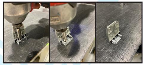
STEP 3: Take second clamp section, add the allen key bolt and position against the first section.
